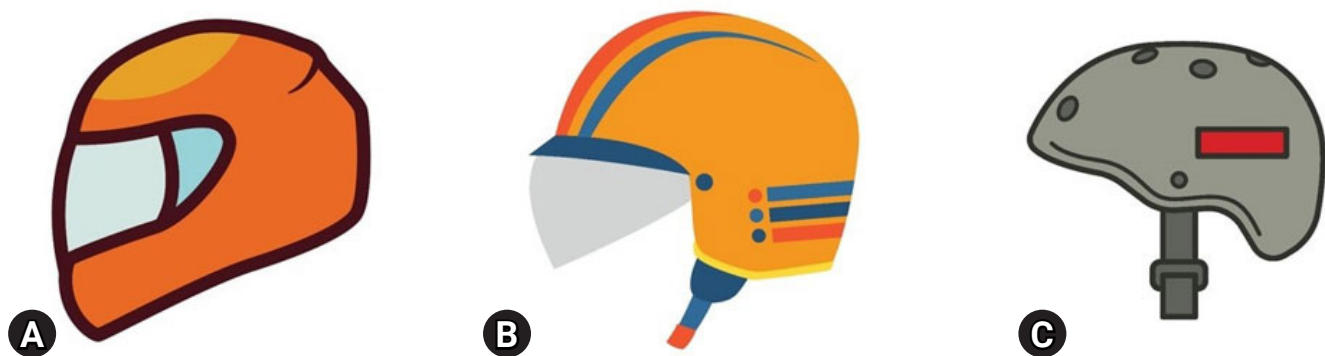
Fig. 1. The different types of helmets. (A) Full-face helmet, (B) open-face helmet, and (C) half-face helmet.
